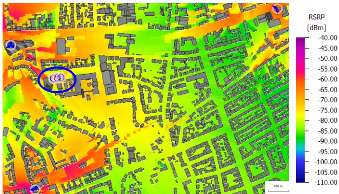
Figure 4: Prediction of the RSRP for 3 deployed macrocells (3 sectors each) and indoor femtocells (blue ellipse) based on a 3D urban vector database
