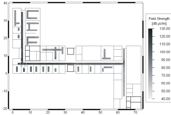
Figure 8: Measured field strength for transmitter Tx 1.
