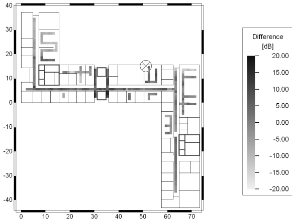
Fig. 15: Difference between prediction and measurement (mean = -0.2 dB, std. dev. = 6.1 dB) for TRX 3
