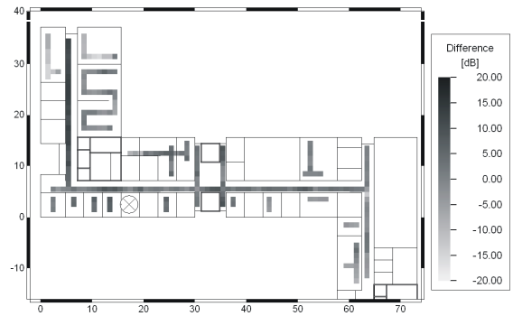
Fig. 14: Difference between prediction and measurement (mean = 1.0 dB, std. dev. = 5.9 dB) for TRX 2
