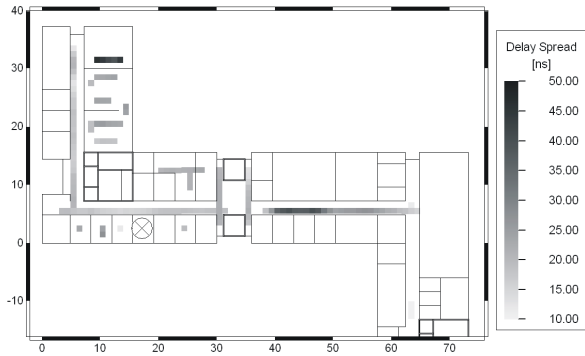
Fig. 12: Measured Delay Spread for transmitter TRX 2
