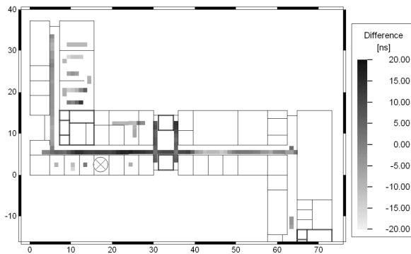
Fig. 16: Difference between prediction and measurement (mean = 0.3 ns, std. dev. = 8.2 ns) for TRX 2
