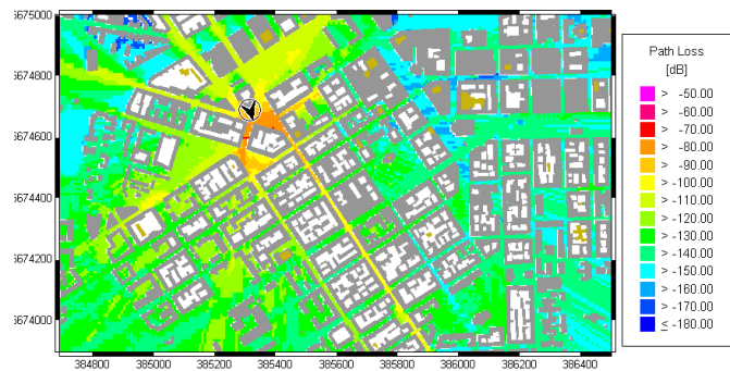
Figure 8. Path loss prediction for “low” BS antenna.
