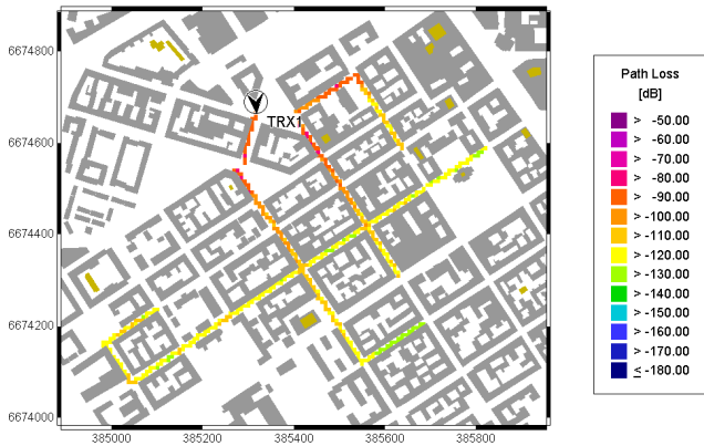
Figure 3. Path loss measurements for "high" BS antenna.
