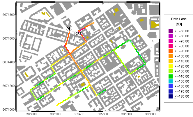
Figure 2. Path loss measurements for "low" BS antenna.
