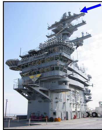
Figure 5: Aircraft carrier island showing yardarm where antenna is mounted.
